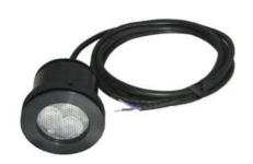
Panel System LED lighting. Anodized aluminum illuminator with 3 power LED and 8°-25°-40° lens. Threaded ring for fastening. Separated external PSU.
